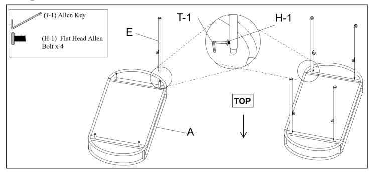
Place the Top Shelf (A) in upside down position on a padded non-marring surface. Insert Legs (E) & Align the hole of Top Shelf (A) with the pre-drilled holes of Legs (E). Secure connection using Allen Bolt (H-1) as shown, tighten it with the help of the provided Allen Key (T-1). Do not yet fully tighten. Repeat same for the remaining Legs(E). Do not yet fully tighten.
