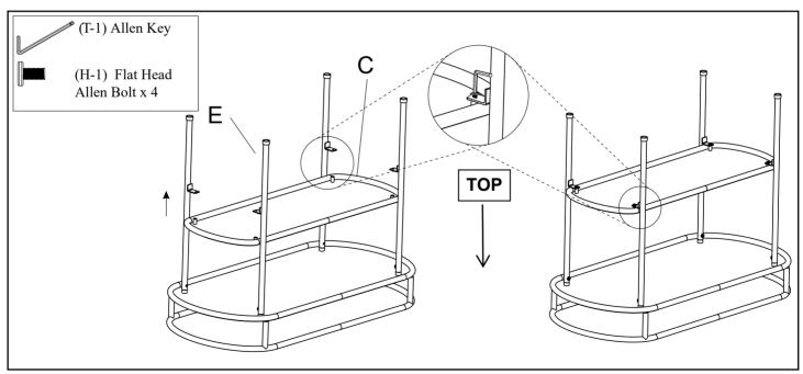
Using a second person to assist you, hold the Middle Shelf (C) upside down against the brackets located on all Legs (E), careful not to scratch any surfaces. While holding, align the screw holes on each component and engage all Allen Bolts (H-1) as shown. Tighten with the provided Allen Key (T-1), but do not yet fully tighten. Once all have been engaged, the Middle Shelf (C) can be let go.
