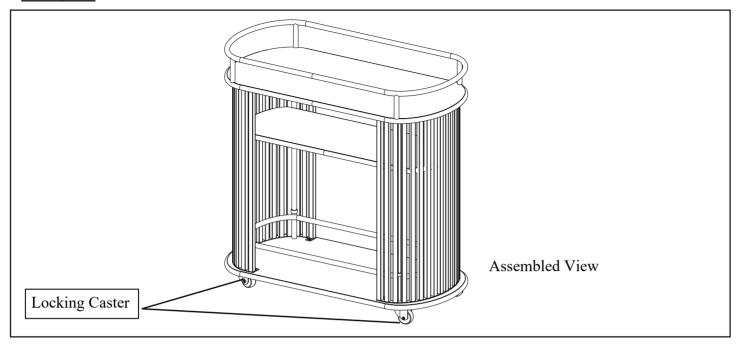
Assembly is now complete and the product is ready for use. Ensure the Locking Casters (G) are engaged when the Bar Cart is stationary. NOTE: Hardware may loosen over time. Periodically check that all connections remain tight and adjust as needed.
