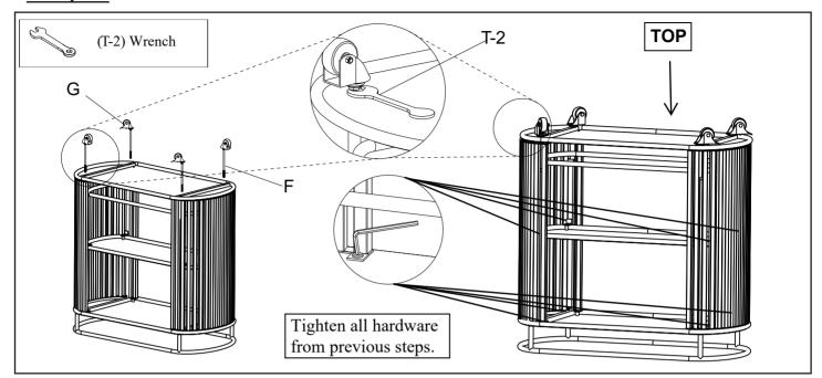
Insert Non-Locking/Locking Casters (F/G) into the assembly as shown. NOTE: it is suggested to install one Locking Caster (G) on each side of the assembly (Left and Right). They will not function as well if they are both on the same side. Using the provided Wrench (T-2), fully tighten all four Casters (F/G). Fully tighten all hardware from all steps. DO NOT OVER TIGHTEN.
