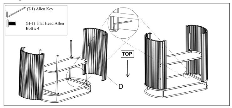
Carefully position the Side Frames (D) with the assembly as shown. Align the holes in the Side Frames (D) with the receiving holes in the Top Shelf (A). Engage all Allen Bolts (H-1) using the provided Allen Key (T-1). Do not yet fully tighten.
