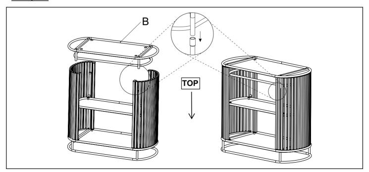
Carefully position the Bottom Shelf (B) onto the assembly as shown. The bottom of the previously assembled Legs (E) have sleeves that the connection tubes of the Bottom Shelf (B) engage with. Ensure all four connection tubes are engaged.
