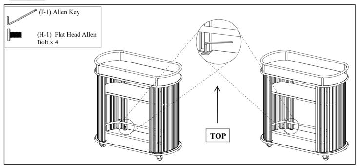
Using a second person to assist you, carefully turn the assembly into the upright position. Align the holes of the Side Frame (D) with the holes in the Bottom Shelf (B). Secure connection with Allen Bolts (H-1) using the provided Allen Key (T-1). Repeat the process for all points of connection. Fully tighten all hardware. DO NOT OVER TIGHTEN.
